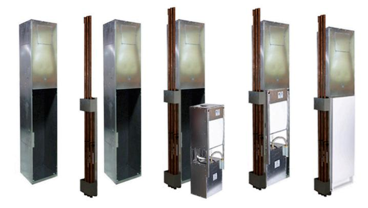
Once the site is clear of any dust and debris, clean and finished, the chassis will ship and is slid into the cabinet. The hoses are attached to the risers, and the electrical cord gets plugged into the outlet.
