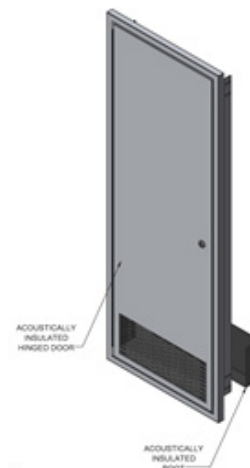
Hinged Return Air Panel with lock, frame, and boot. Requires a minimum 2" base extension (Option 90)
