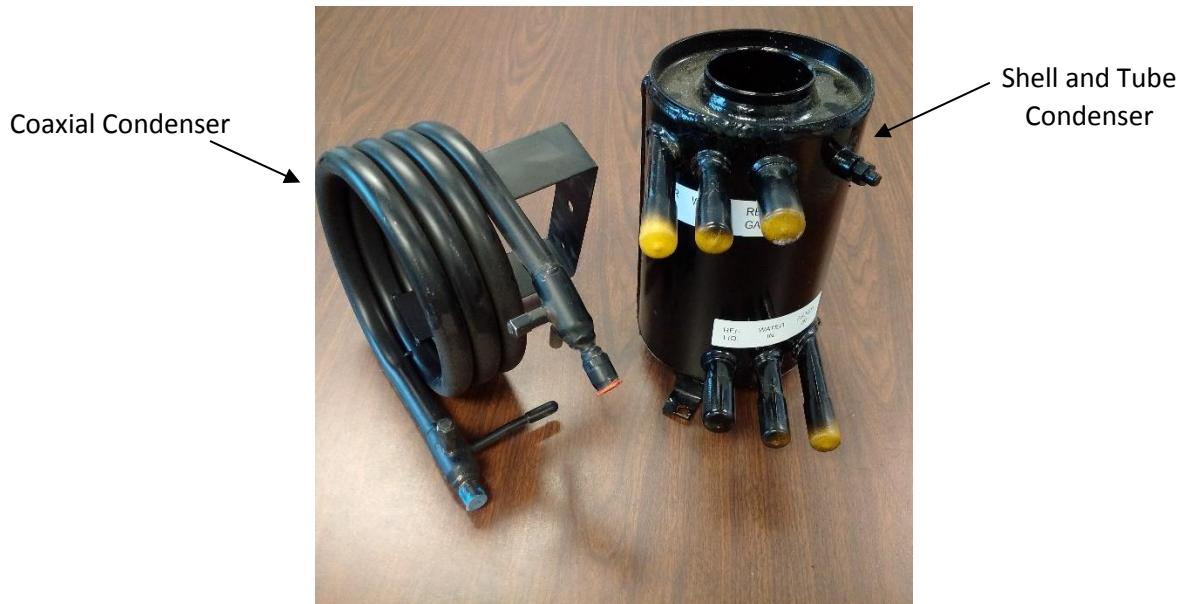
All manufacturers of regular WSHP use the heat exchanger on the left. It's a coaxial condenser and must also operate as an evaporator in the heating mode. The Bulldog is optimized for cooling mode only by utilizing a more effective condenser – the shell and tube on the right.
