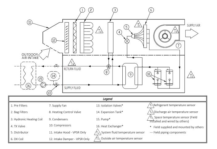
The fan runs continuously when the unit is enabled. The intake damper (when equipped or by others) is signaled to open prior to the fan starting.
