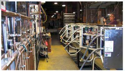
Every single **BULLDOG** is tested for refrigerant leaks 6 times and undergoes a factory run test.
